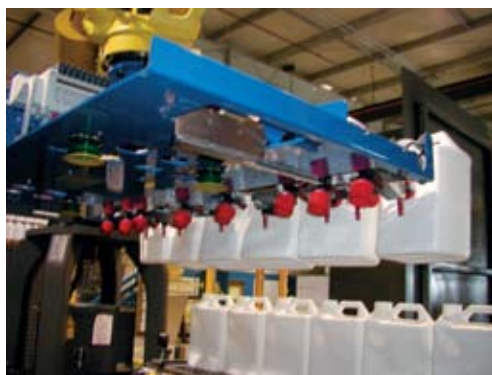
Figure 10. Sample Pet Food Container Depalletizing Equipment
